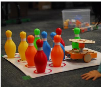
With a masking-tape lane and some plastic pins, KIBO can become a [programmable bowling ball](#). Kids can plan a program that will send KIBO down the lane, measure the results, and tally the number of pins knocked down.
