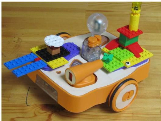
The [Building Brick Extension Set](#) connects KIBO to the world's most popular building bricks, including LEGO®. Building brick plates attach to KIBO's module sockets or to the stage art platform, allowing kids to build onto KIBO in spectacular ways. Letting kids decorate and personalize KIBO has always been central to our philosophy, and the "BBES" takes that to a whole new level.
