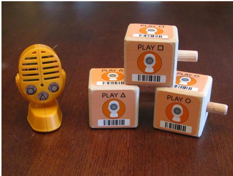
The new module looks like an old-fashioned microphone in front and a speaker in the back, and it plugs into any of KIBO's module sockets. Kids can record up to three different sound clips, then program KIBO to play back the sounds using three included programming blocks.
